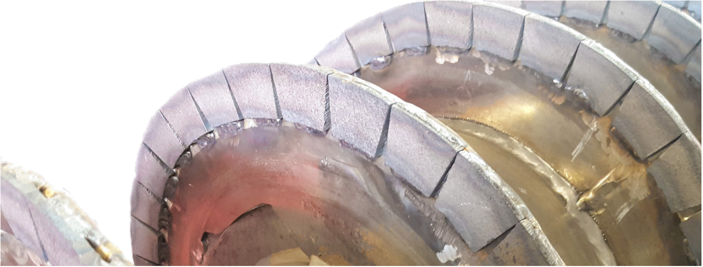
Decanter centrifuge fitted with Ferobide tiles
